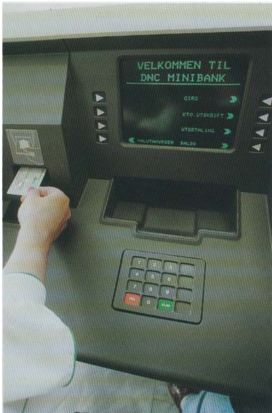
Figure 2 The most common and frustrating problem for all users of mini-banks (automatic tellers to some) and similar technology, is to insert the card in the correct orientation. By putting a tactile marker on the card, it will be much easier to turn the card to the proper orientation before inserting it in the card-reader. This will not only make the service both simpler and friendlier to users, but may be essential to blind and visually impaired users
