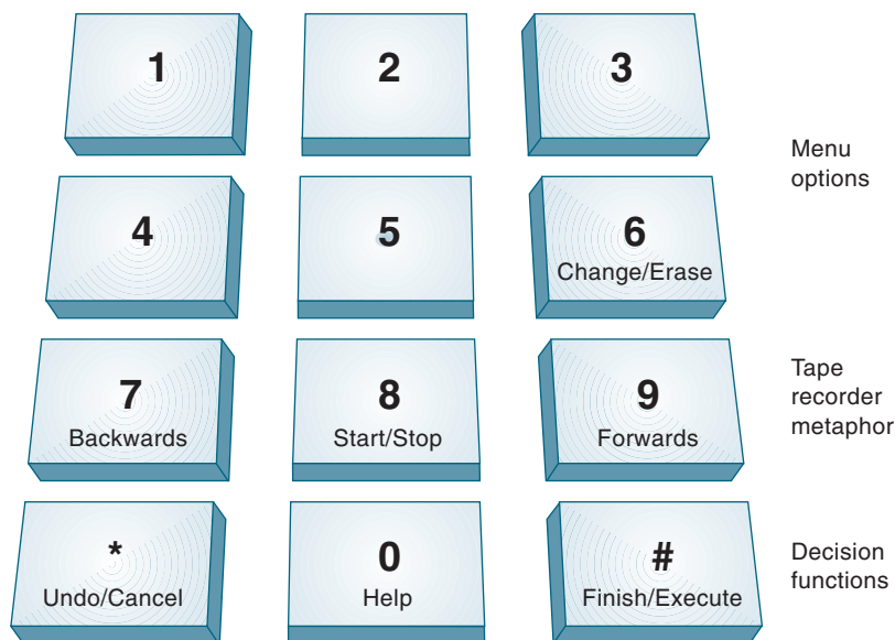
Figure 3 A common functional keypad interface proposed by Telia for all kinds of interactive voice response services: Keys 1–5 for menu options; key 6 = change/erase; keys 7–9 for the 'tape-recorder' metaphor (key 7 = fast rewind, key 8 = stop/start, key 9 = fast forward); and keys * 0 # for decision functions (* = undo/cancel, 0 = help, and # = finish/execute) (after [10])
