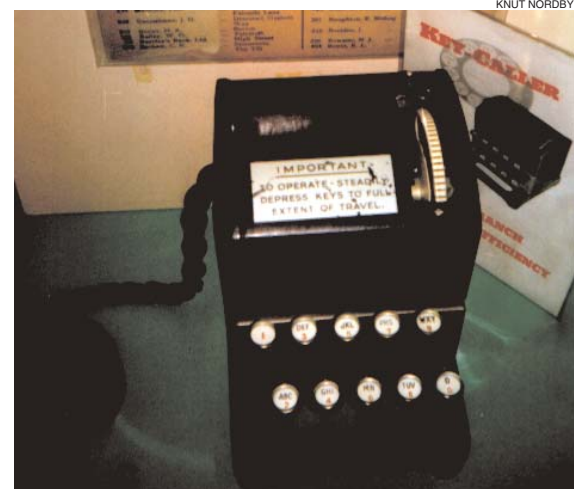
Figure 4 British (General Post Office) push key number dialler. This device was used in exchanges to alleviate the physical strain on operators who had to dial telephone numbers all day on a rotating dial
