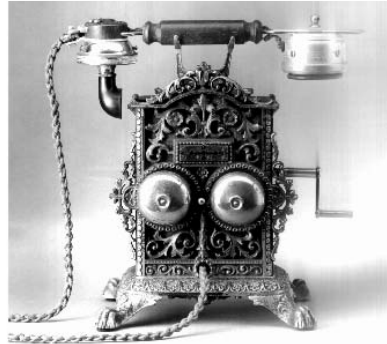
Figure 1 Norwegian telephone set from 1893 with inductor crank. This telephone set worked with the simple user interface from the early days of telephony. The earpiece on the handset can be moved to adapt to 'small and large heads', a simple ergonomic concession to user variability
