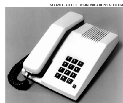
Figure 5 'Tastafon', the first Norwegian 'touch-tone' push-button (DTMF) telephone from 1981. Push buttons are much easier to operate than a rotating dial. Note the inverted layout of the number keys which does not follow ITU-T Recommendation E.161
