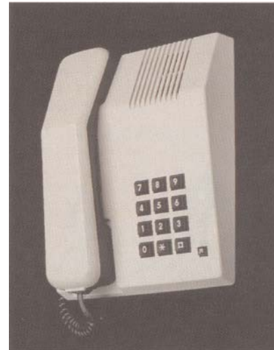
Push buttons and multi frequency signalling was the key to a multitude of new telephone services. "Tastafon" was developed in the late seventies and introduced in 1981
