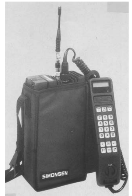
Figure 4 The first automatic mobile telephones of the NMT system were more portable than “handy” unless installed in a car. The picture shows an early NMT-900 from the Norwegian manufacturer Simonsen
