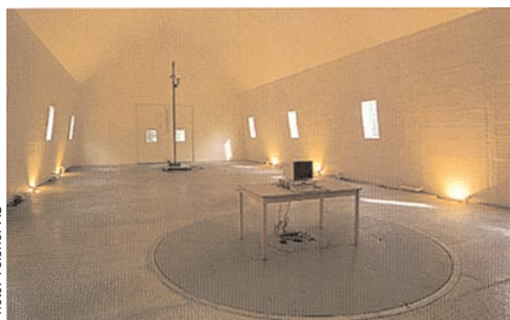
Figure 2 OATS interior, 3 and 10 metres measuring sites with weather protection
