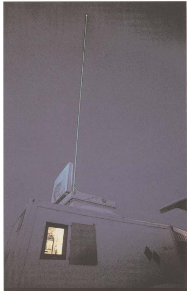
Lidar measurements carried out by the German Koldewey Station. These measurements give vertical profile information on particles and ozone from 10–40 km in the stratosphere
