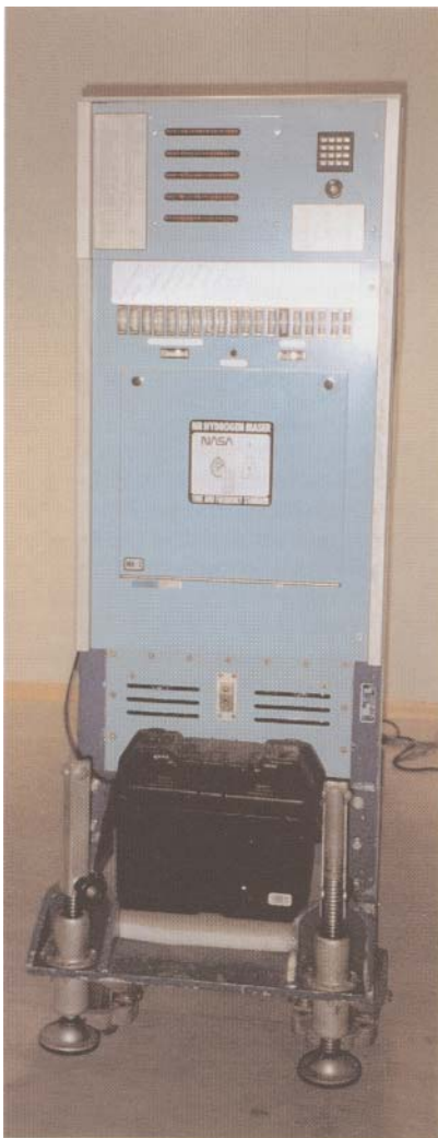
Figure 7 Hydrogen maser frequency standard (atomic clock) used to provide reference signals to the data acquisition electronics
