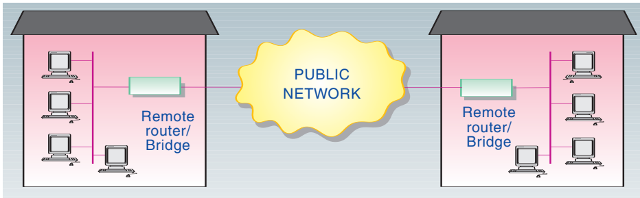
Figure 1 Two LANs interconnected via routers/bridges and leased lines
