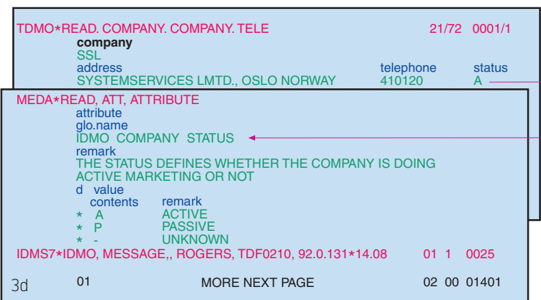
Figure 3 Figure (a) shows an ordinary alphanumeric picture from DATRAN. Figure (b) depicts the standard layout of a DATRAN picture. Figure (c) shows how data relate to each other. Figure (d) shows a Help screen for a specific field, provided by direct access to MEDA. The many pre-made dialogue features of DATRAN are not illustrated
