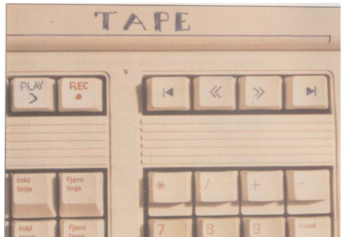
Figure 4 (Left) Close-up of console screen, showing interaction buttons, slide bar, and peak meter for the simulated tape recorder; (right) showing tape functions accessible from the computer keyboard, without using the mouse
