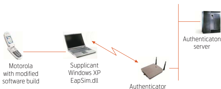
Figure 10 Test-bed architecture used for testing the EAP-SIM authentication
