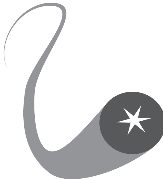
Figure 5 A telecom fiber is a thread of glass, slightly thicker than a human hair. The beam of invisible infrared light guided along the center of the thread has a diameter of 0.01 mm
