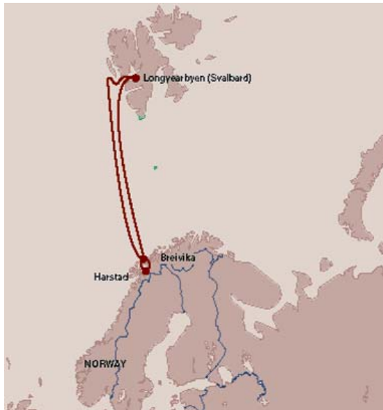
Figure 6 (From [6]) Two separate optical cables connect Svalbard to mainland Norway
