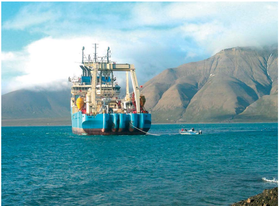
Figure 1 In January 2004, a submarine optical cable between Svalbard and mainland Norway was opened. The photograph shows the cable ship as it starts its cable laying operation from Svalbard in July 2003. Submarine cables are major engineering projects, where the entire cable and accompanying signal regenerators are made in a factory, before they are taken on board a cable ship
