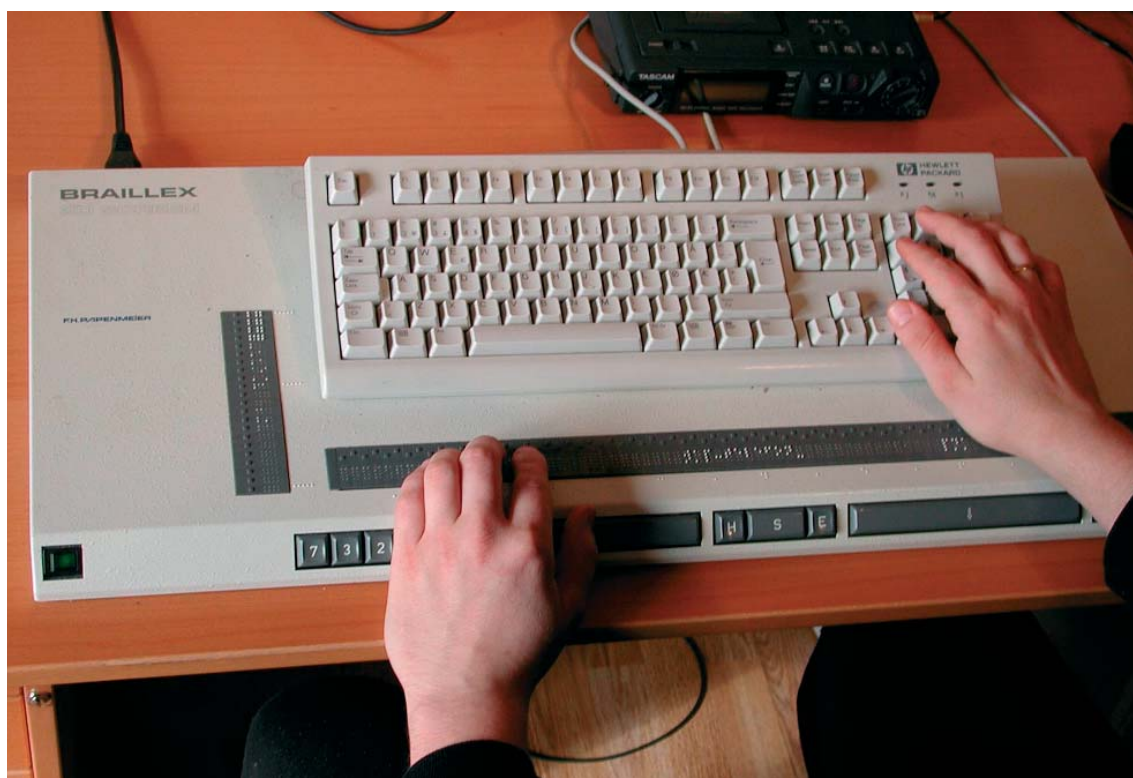
Figure 1 The Braille tactile display is usually placed under the normal PC keyboard.
