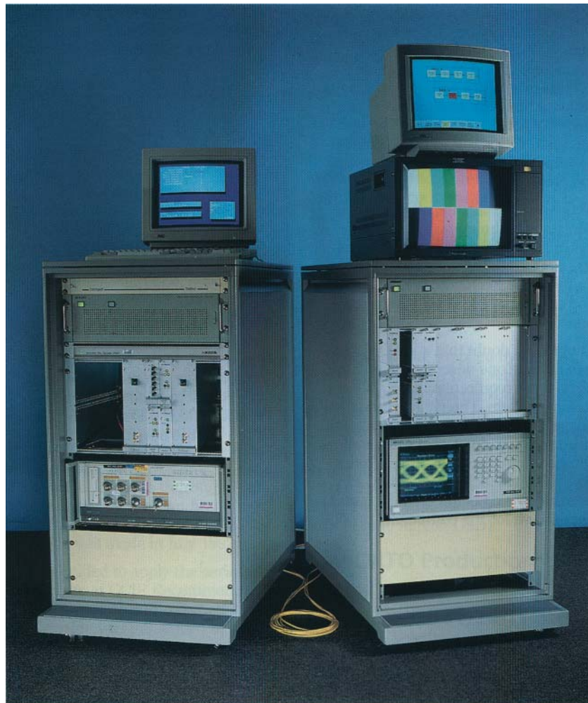
Figure 14 OIU (Optical Interface Unit) (picture taken at a demonstration in Brussels in 1993, reproduced by permission from GEC Marconi)
