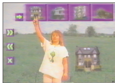
Figure 7 Using the Mandala system the user's body is projected into a virtual world in which she can interact
