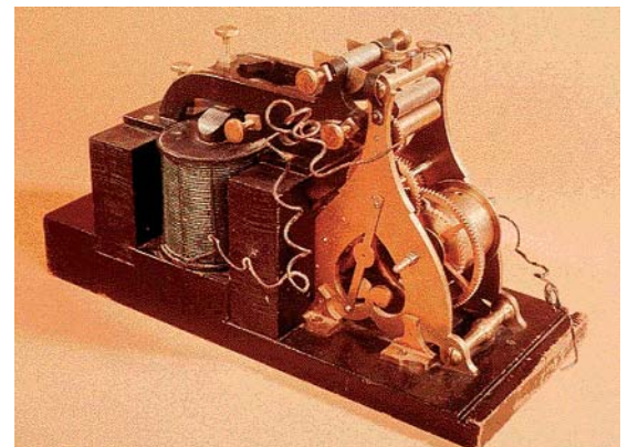
In 1844, Morse demonstrated to the US Congress the practicality of the telegraph by transmitting the famous message "What hath God wrought" over a wire from Washington to Baltimore. The picture shows Morse's telegraph receiver, which he used at the demonstration in 1844 (Smithsonian National Museum of American History)
