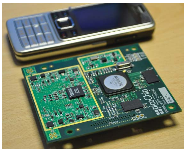
Figure 5 picoChip system module for embedding of femtocells into third party products like set-top boxes and home-gateways. Source: picoChip
