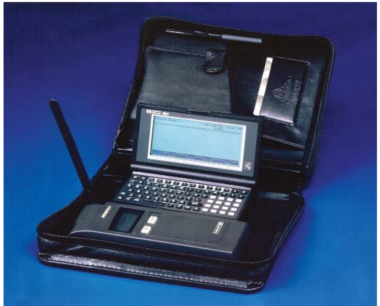
Figure 1 A wireless e-mail solution based on Mobitex. The Ericsson 'Viking express' from 1992 consisting of the Ericsson Mobidem together with an HP-95 palmtop and bundled with Research in Motion's (RIM) MobLib-Plus application programming interface (API) to work with major e-mail systems. (Source: http://blackberryplanetbook.com/index.php/Image:Mobidemhp.jpg )
